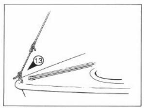
Secure the mast in the upright position by attaching the forestay to the bow plate, as shown. (Fig 13) .
