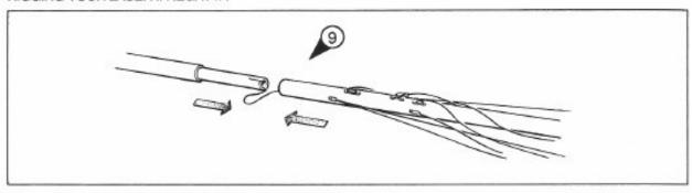
\* Take the top mast section (Part B) and slide into bottom mast (Part A) making sure the luff (groove is in line and the sleeve is fully pushed home. (Fig 9) 4.
