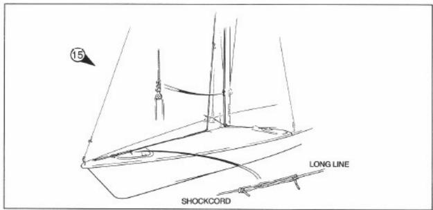
Attach the spinnaker pole uphaul/down haul line as shown, (Fig 15) A.
