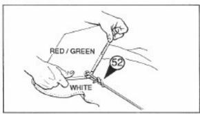
\* Attach the spinnaker downhaul line to the recovery patches on the inside of the spinnaker as shown. (Fig 53) .
