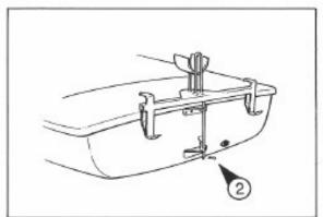
\* Detach rear mast support (if fitted) by removing 'R' clip
