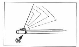
Take the clew tie down (Part P), pass it through the clew eye, around the boom twice, as shown, (Fig 36) ➤, finishing with a reef knot or similar.
